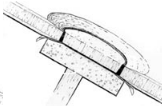
Figure 5-14 Brace a temporary backing against the back of the hole to support the new core.
