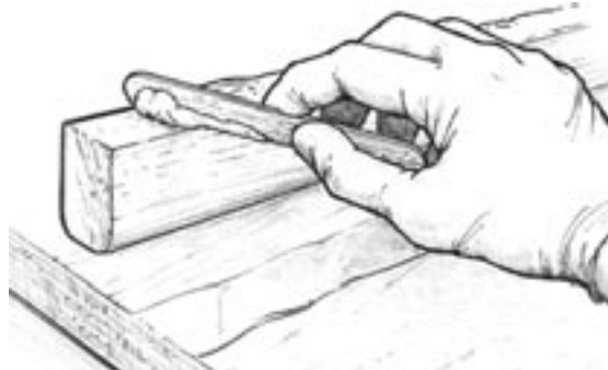
Figure 9-9 Apply enough thickened epoxy to one of the bonding surfaces so that a small amount will squeeze out of the joint when clamped with moderate pressure.
