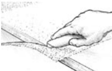
Figure 9-17 Trim excess cloth after the epoxy has begun to gel using a sharp utility knife.
