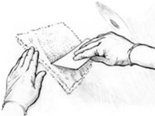
Figure 4-3. Smooth the wet-out fabric against the waxed panel to laminate a backer that matches the panel contour.
