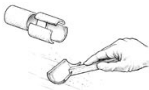
Figure 9-24 Tip off the fresh coat of epoxy with the grain, using a foam roller brush to remove bubbles and roller marks.
